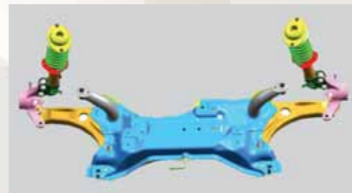
Frame type front suspension system for smoother drives
